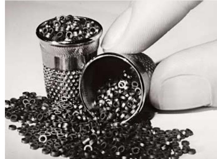
*Tiny washer-shaped ferrite cores were the heart of memory technology at the time.*
