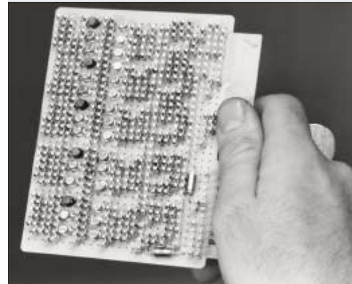
*SMS, or Standardized Modular System, technology replaced vacuum tubes.*
